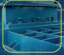
Adjustable Shear Beam – The body shear blades are adjustable from the exterior of the machine.
